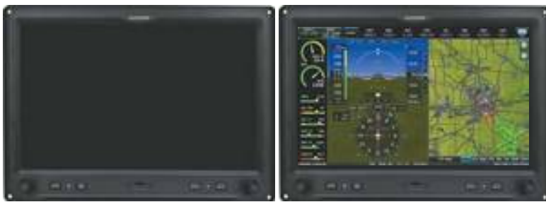
G3X Touch Full-Screen Reversionary Mode (Failed PFD)
