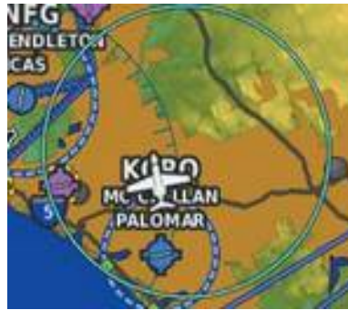
Navigation Map - Glide Range Ring (Ideal Descent Profile - Wind 245° at 25 kts)
