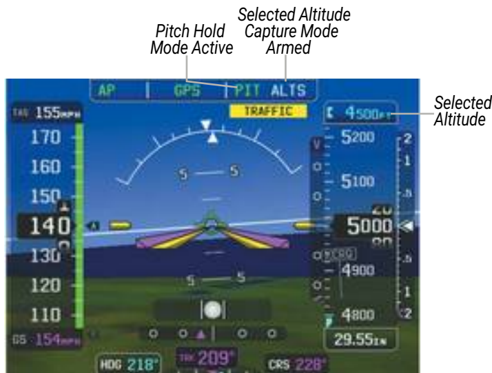
Pitch Hold & Selected Altitude Capture Modes
