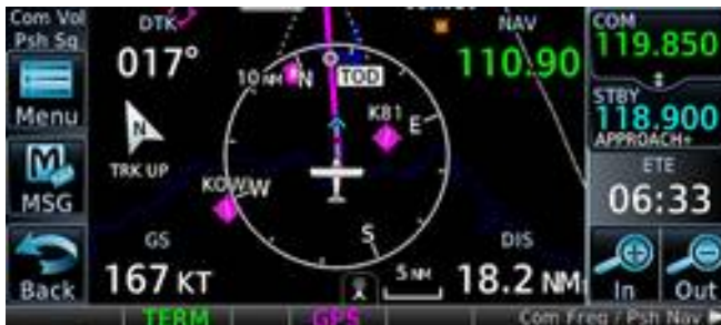
Top of Descent Indication (GTN) Garmin G3X TouchPilot's Guide for Certified Aircraft
