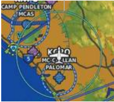
Navigation Map - Glide Range Ring (Ideal Descent Profile - No Wind)
