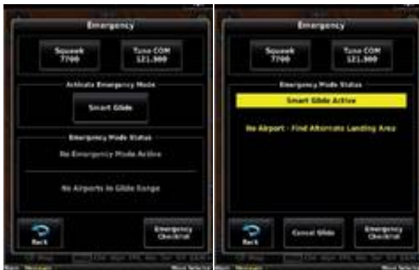
Airport Not Within Range (Smart Glide Not Active)
