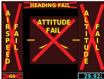
Figure 1-2 G5 PFD Page Failure Annunciations
