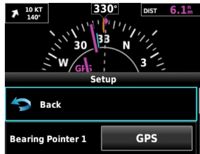
Figure 2-20 Bearing Pointer Setting
