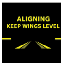
Figure 1-5 Attitude Aligning Keep Wings Level Indication
