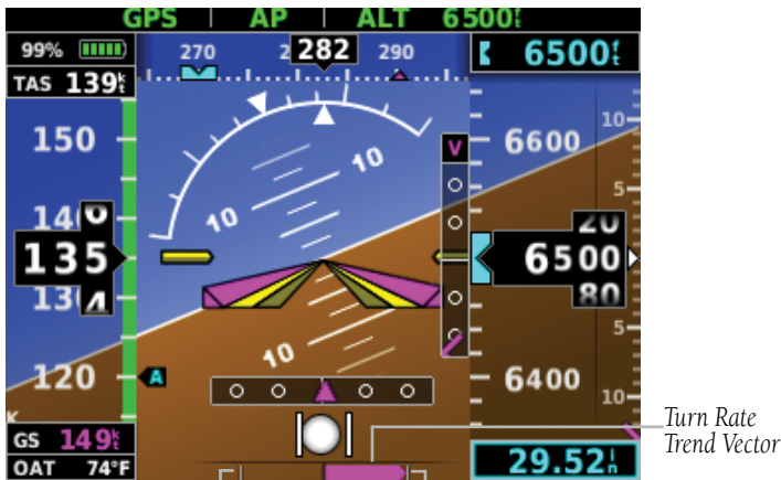
Turn Rate Indicator (Standard Rate Tick Marks)
