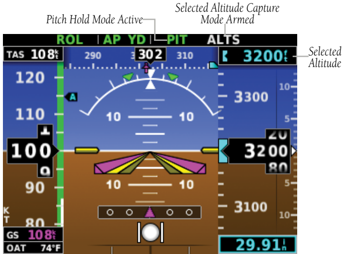
Figure 3-8 Pitch Hold & Selected Altitude Capture Modes
