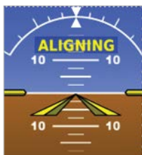
Figure 1-4 Attitude Aligning Indication
