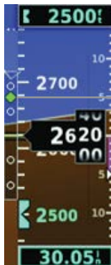
Figure 2-24 Vertical Deviation Indicator (Glideslope ILS Source) - PFD
