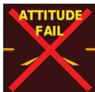
Figure 1-6 Attitude Failure Indication
