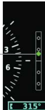
Figure 2-25 Vertical Deviation Indicator (Glideslope ILS Source) - HSI
