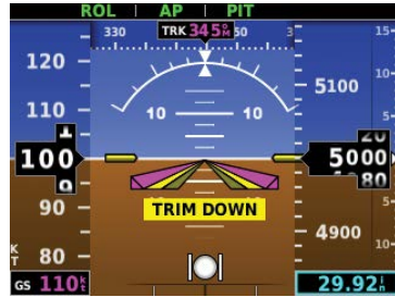
Figure 3-22 TRIM DOWN Alert
