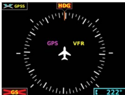
Figure 1-3 G5 HSI Page Failure Annunciations
