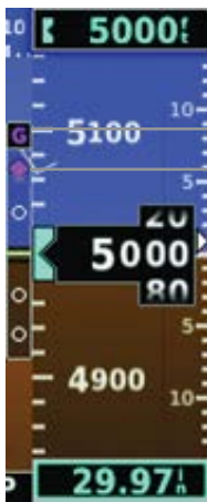
Figure 2-26 Vertical Deviation Indicator (Glidepath GPS Source) - PFD
